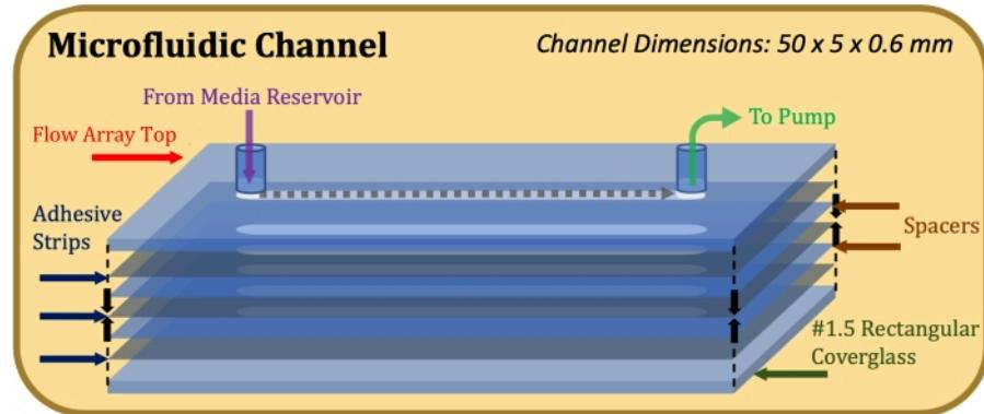
**Figure 1: Exploded-view schematic of the microfluidic channel construction.** The top element is the top portion of the flow array, thin grey elements are adhesive strips, thin blue elements are mylar spacers, and the bottom element is the rectangular coverglass. [Please click here to view a larger version of this figure.](#)
