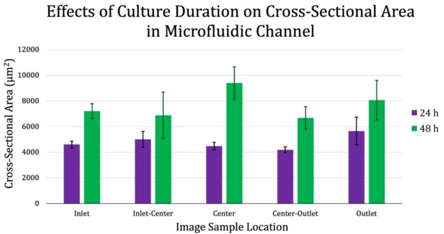
**Figure 5: Graphical representation of the data collected during the 24-48 h microfluidic channel imaging experiment.** This includes six cross-sectional area samples from each of five locations along the relevant length of the microfluidic channel (as depicted in Figure 2). Error bars represent standard deviations. [Please click here to view a larger version of this figure.](#)
