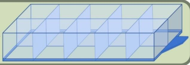
**Figure 3: Diagram of the eight-well chambered coverglass used for the fixed-well culture, staining, and imaging experiment comparing the effects of initial cell seeding density and culture duration on the formation of cell layers.**
