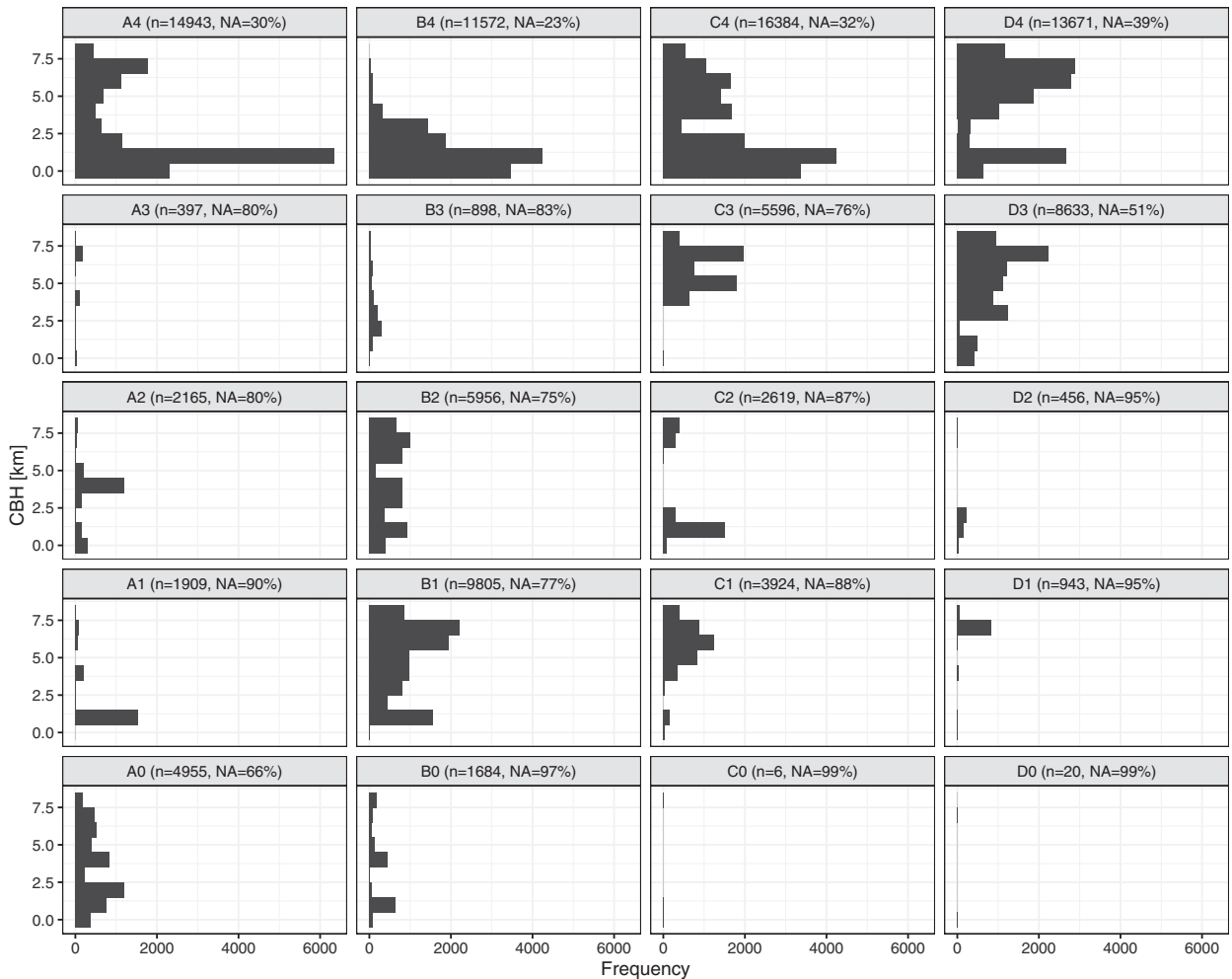
FIG. 8. Frequency distribution of lowest cloud-base height for the clusters shown in Fig. 5. The CBH measurements are sampled only for the periods when the cluster was present for 10 min or longer. On average, around 75% of the CBH are reported missing because of the clear-sky conditions and low signal-to-noise ratio. The valid CBH observations in each cluster ( n ) and the percentage of missing CBH measurements (NA) are given at the top of each panel.
