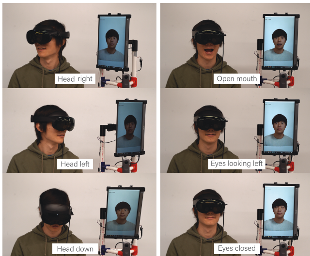
Figure 3: Several examples of head rotation, facial expression, and eye gaze. The system replicates the VR user’s head rotation through an articulated display and their facial expression & eye gaze through an avatar animation.
