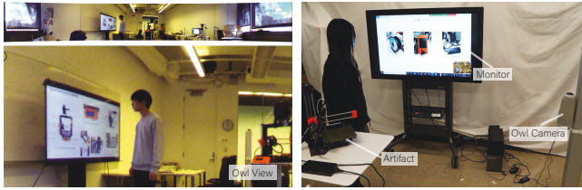
Figure 9: A typical view of Owl system that provides a wide angle and zoomed images of the room (Left) and setup for the Owl condition (Right).
