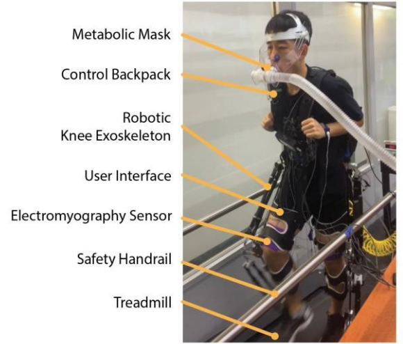
Fig. 1. Experimental setup for validating the PMC controllers.
