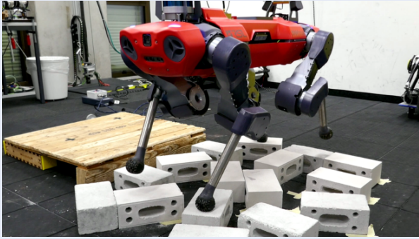
FIGURE S11 ©2021 IEEE. CBF safety filter on a quadruped. A multilayered safety filter design is used that integrates predictive safety filters with CBFs to ensure safe foot placement on viable footholds while maintaining system stability. CBF constraints are integrated into both a mid-level predictive filter and a low-level CBF based filter given by (26), ensuring a consistent safety specification across planning and control layers [103].
