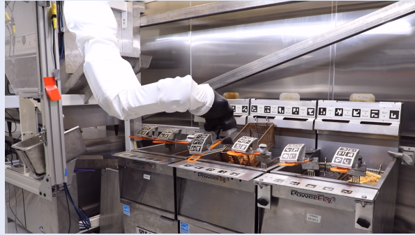
FIGURE S13 ©2022 IEEE. CBF safety filter on a robotic arm in an industrial kitchen. Maintaining safety in a dynamic work environment shared with human personnel requires online modification of arm reference trajectories, but directly recomputing trajectories online is computationally intractable for real-time operation. CBF-based safety filters are used to efficiently modify trajectories given ongoing changes in the environment. [101].
