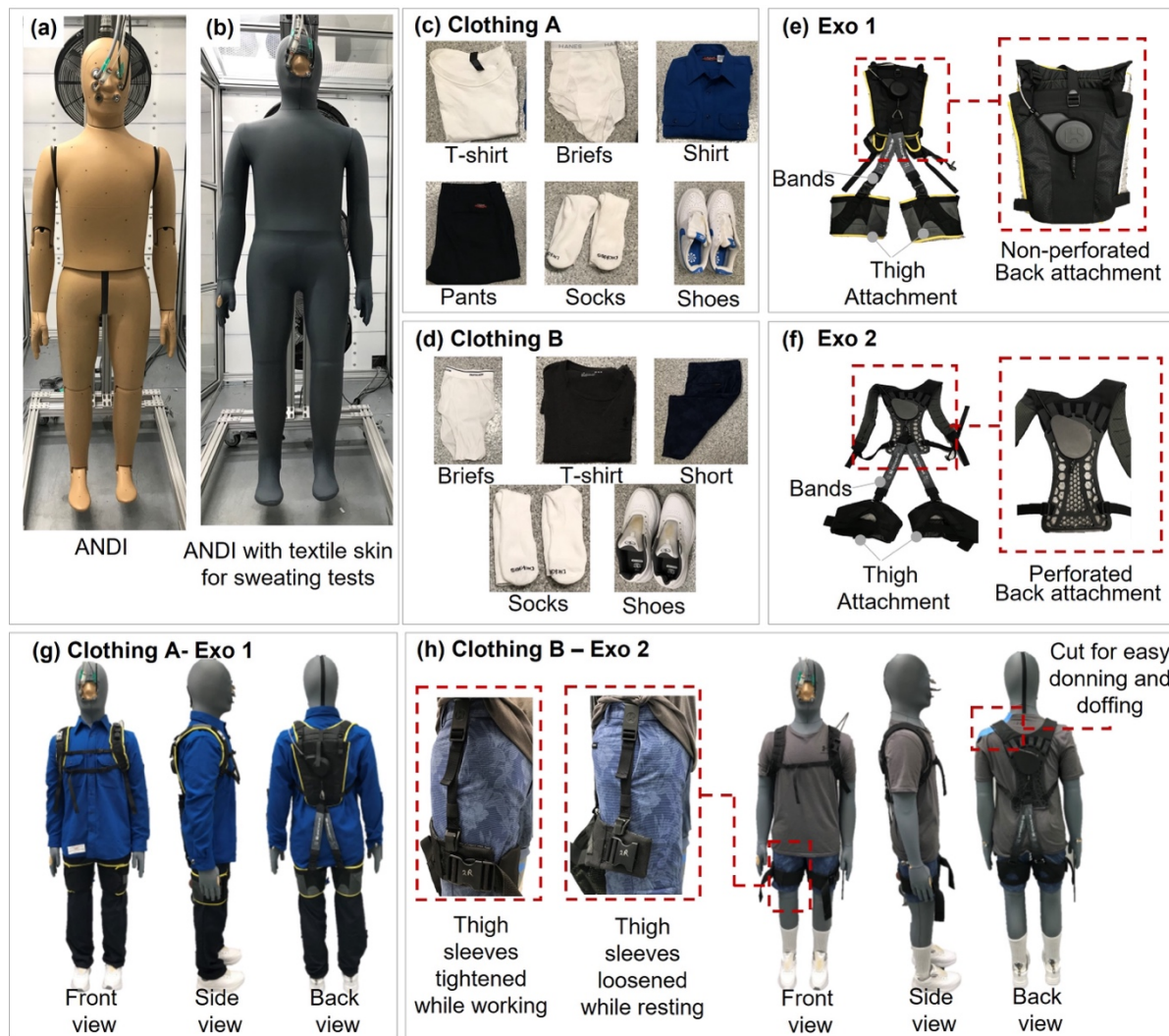
Figure 1. (a) Thermal manikin ANDI in the nude and (b) wearing textile skin to spread the sweat (water) uniformly over its surface; the clothing ensemble (c) "A" (full length) and (d) "B" (summer); exosuits (e) "1" (Apex 1: "Exo 1"), (f) "2" (Apex 2: "Exo 2"); and example of ANDI wearing (g) the Exo-1 and clothing ensemble A and (h) Exo 2 with clothing ensemble B.
