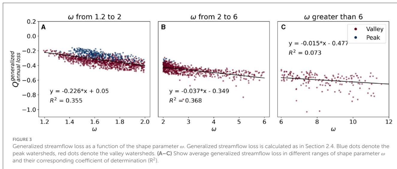
shape parameter of the valley watershed (an average value of 3.1) than the peak watershed (an average value of 1.3). When comparing with the streamflow loss in dry years relatively to normal years, the shape parameter ranges from 1.2 to 2 and from 2 to 6 correlates well with  $R^2$  of 0.355 and 0.368, respectively. The shape parameter
