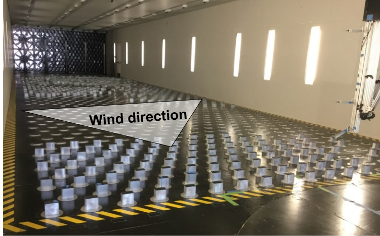
Fig. 4. Implementation of complex heterogeneous terrain in Terraformer, specifically Site 8, in a 1:100 scale based on Fig. 3 (a-j).
