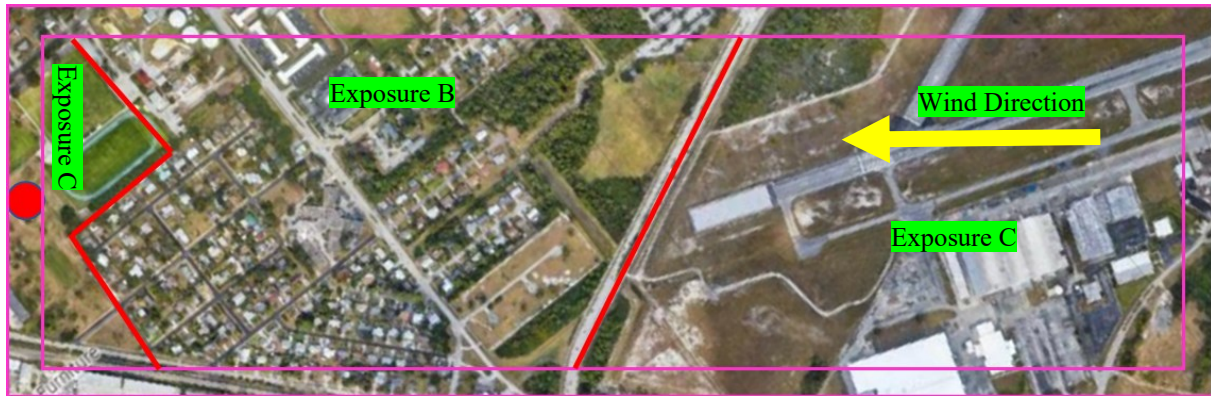
Figure 1 Example of sites with different land coverages, especially with a complex immediate upwind; it is not straightforward to decide about the exposure when there is a complex terrain (Exposure B(suburban areas) and Exposure C (open terrain, airport) are based on ASCE/SEI7-16 (2017))
