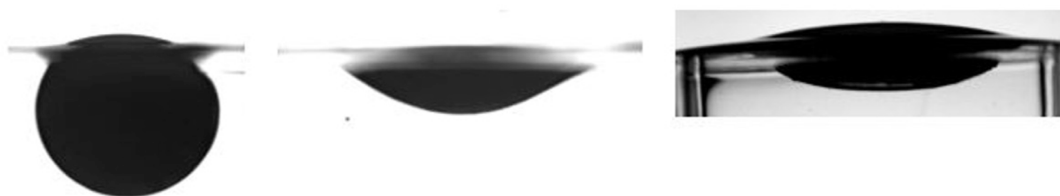
Figure 5. Examples of droplets of GB suspensions on hexadecane: GB-0 ellipsoid (left), GB-0-s half ellipsoid (middle), and GB-GH-s ellipsoid (right).
