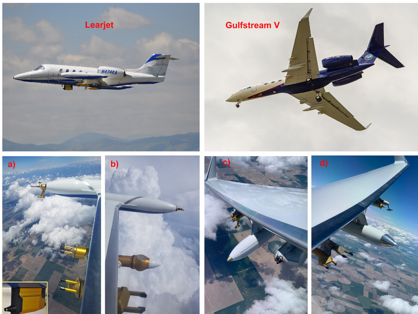
Fig. 1. Instruments installed on the (left) Learjet and (right) GV for the SPICULE project. (a) Learjet right wing: AIMMS-20 and FCDP in tip tank, 2D-S and 2D-Gray probes on pylon. Hawkeye installed on bottom of fuselage shown in inset. (b) Learjet left wing: FFSSP in tip tank, KPR radar and HVPS on wing pylon. (c) GV right wing: 2D-C, 2D-S, FCDP, HCR radar, and Hawkeye. (d) GV left wing: CDP, PCASP, HOLODEC, and HVPS [photo credits: Learjet: Code10 Photography; Gulfstream V: Pavel Romashkin; panel (a):Ted Fisher; panel (b):Sarah Woods; panels (c) and (d): Kyle Holden].
