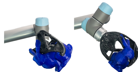
Fig. 10. Post-grasp stability test for the bunny. We measure the maximum roll angle both CW and CCW (left) and forward tilt angle (right) before the bunny falls.
