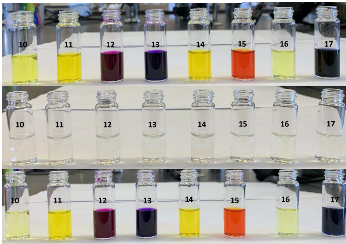
Fig. 2. Photographs of 6-aryldibenzo[b,d]pyrylium salts 10–17 in solution. Top: Vials containing 2 mL solutions of 10–17 , 1.0 mM in CH 3 CN. Middle: Vials from the top after addition of 40 µL of TEA. Bottom: Vials from the middle after addition of 120 µL of TFA.
