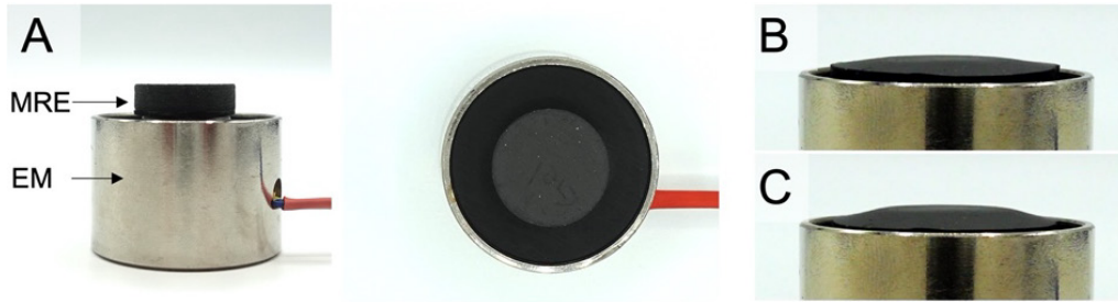
Figure 1. (A) Magnetorheological elastomer interface (20 mm diameter, 5 mm thick) sitting atop the electromagnet (EM), (B-C) vibration observable through shape change at 2Hz with a thin MRE sample (17 mm diameter, 1 mm thick).
