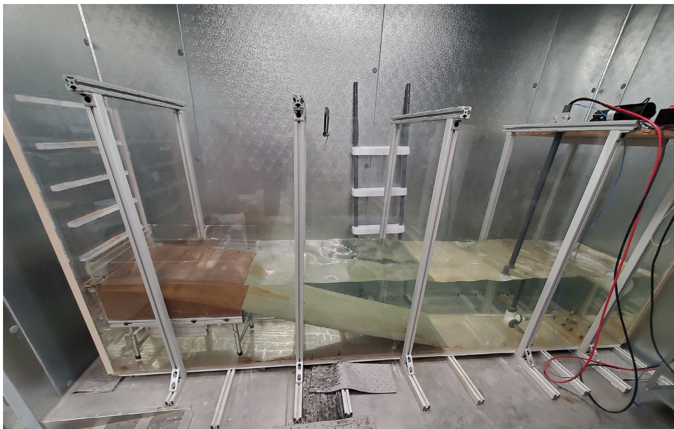
FIGURE 3 Side profile of the wave tank device. To the left of the photo is the beach ramp and the sediment beach. On the right side of the photo is the plunging wave generator and a heating element. When the tank is in use cameras are mounted to the overhead aluminum struts. The wave tank is located within a large walk-in freezer. The wave tank is 3 m long \times 0.6 m wide \times 1.2 m tall.
