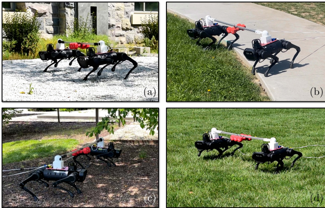
Fig. 19. Snapshots demonstrate the proposed layered controller's performance for a series of cooperative locomotion experiments. Outdoor experiments: (a) cooperative locomotion on gravel, (b) transitioning from concrete surface to grass, (c) cooperative locomotion on mulch, and (d) cooperative locomotion on grass. The robots cooperatively transport a payload of 4.53 (kg) (36% uncertainty) in (b) and (c) and 6.80 (kg) (55% uncertainty) in (a) and (d). Here, (a) and (c) show the snapshots where the distributed MPC is adopted, while (b) and (d) show the snapshots where the centralized MPC is employed.
