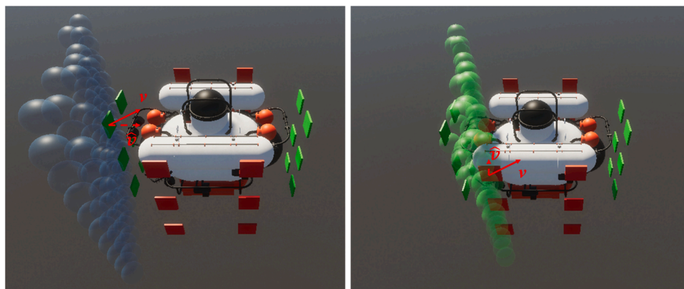
Fig. 5. Example of virtual sensor intensity in DT module: normal vector for intensity calculation.
