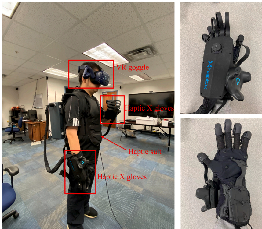
Fig. 6. User setup with HTC Vive, haptic suit, and haptic gloves.
