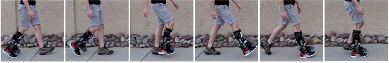
Fig. 10. Assisted mobility with model predictive interaction primitives running in real-time on a SpringActive Ruggedized Odyssey prosthesis.
