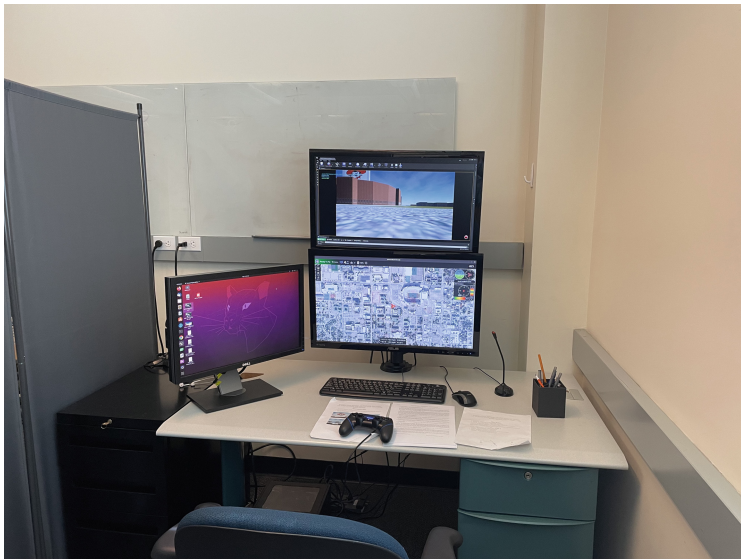
Fig. 3. Experimental setup: upper screen shows the environment and the lower screen shows the ground control station. Participants are also required to use the mouse and the joystick.
