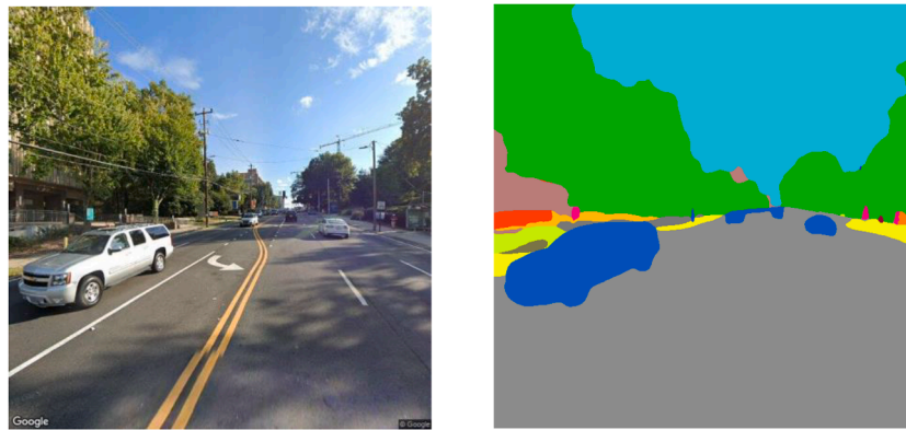
Fig. 2. Street View image from Google API (left) and the result of image parsing using PSPNet (right).
