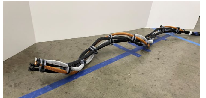
Fig. 5: The physical model of the HISSbot with one actuator pressurized, showing a similar helical structure to the constraint model seen in Fig. 3(b).
