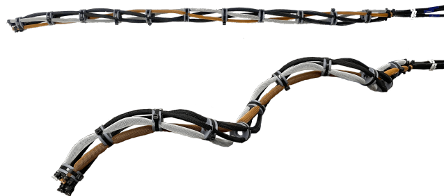
Fig. 1: The HISBot uninflated (top), and pressurized to form a helical shape for sidewinding (bottom). Cyclical contraction of the four McKibben actuators produces locomotion via a twisting-helix motion.
