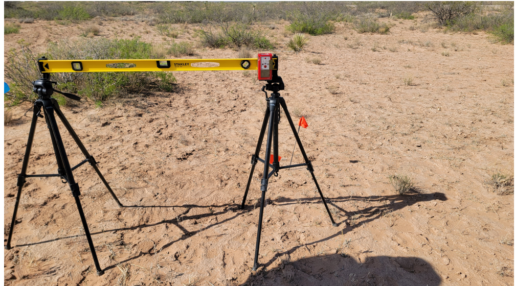
Figure 4. Photo of the surface roughness measurement device.
