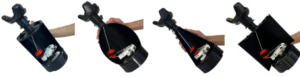
Figure 4: Location of the active mass which corresponds to the location of CoG when a user performs the same action across four different shape shells. (From left to right) cylindrical, spherical, conical, cuboid
