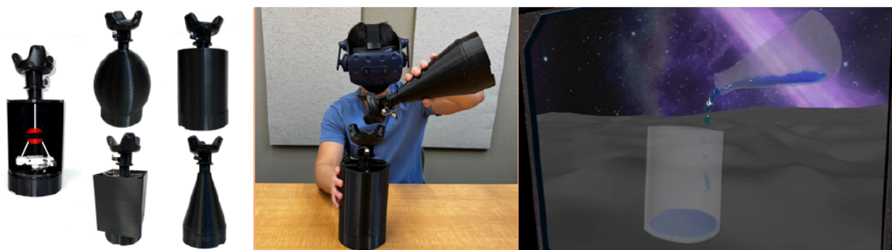
Figure 1: Geppetteau uses a string-based pulley system to dynamically relocate a vessel's center of gravity, producing haptic sensations of virtual fluids. Geppetteau can augment everyday vessel profiles, e.g., 4 example vessel shapes shown (left). Users at any physical setting (middle) can interact with virtual fluids in virtual settings (right).
