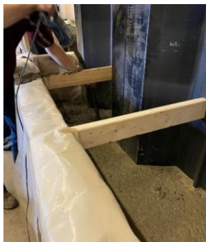
Fig. 12. Concrete poured around specimen.
