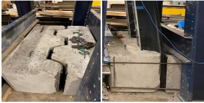
Fig. 16. Restraining structure with elastomeric padding.
