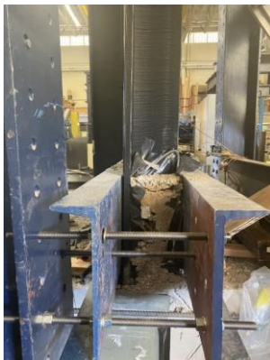
Fig. 18. Increased embedment depth with two channels.
