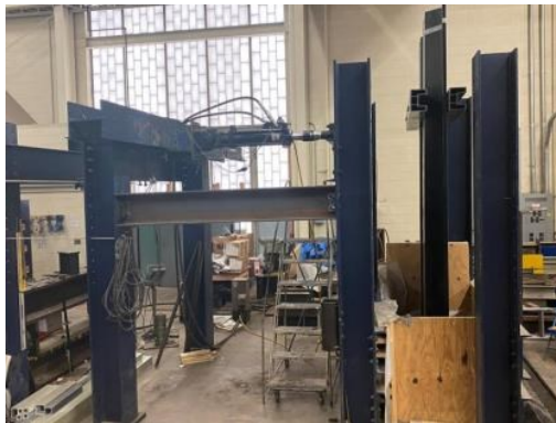
Fig. 5. Sheet pile test set up with Actuator.
