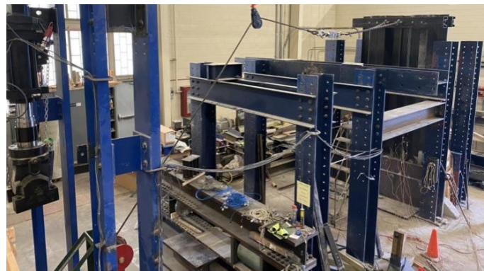
Fig. 6. Sheet pile test set up with Winch.
