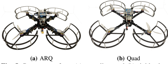
Fig. 5: Prototypes of our (a) compliant and (b) rigid robots.
