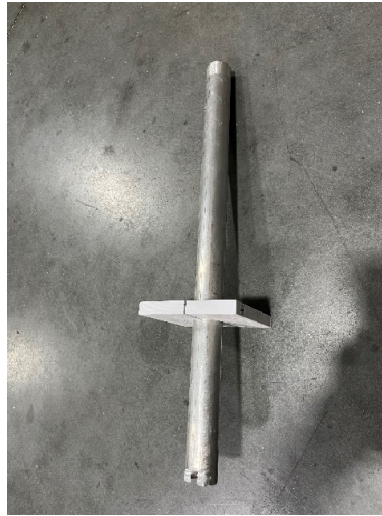
(b) Aluminum rod with plastic collar.
