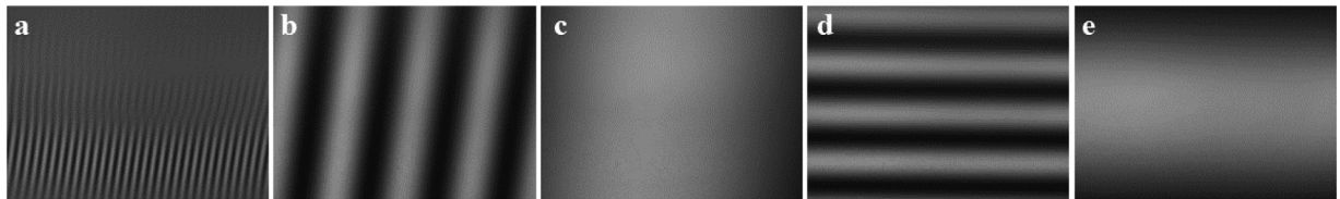
Fig. 6. Examples of our captured fringe images. (a) One of the 9-step high-frequency vertical fringe images with a period of 18 pixels. (b) One of the 3-step middle-frequency vertical fringe images with a period of 144 pixels. (c) One of the 3-step low-frequency vertical fringe images with a period of 912 pixels. (d) One of the 3-steps middle-frequency horizontal fringe images with a period of 216 pixels. (e) One of the 3-step low-frequency horizontal fringe images with a period of 1140 pixels.
