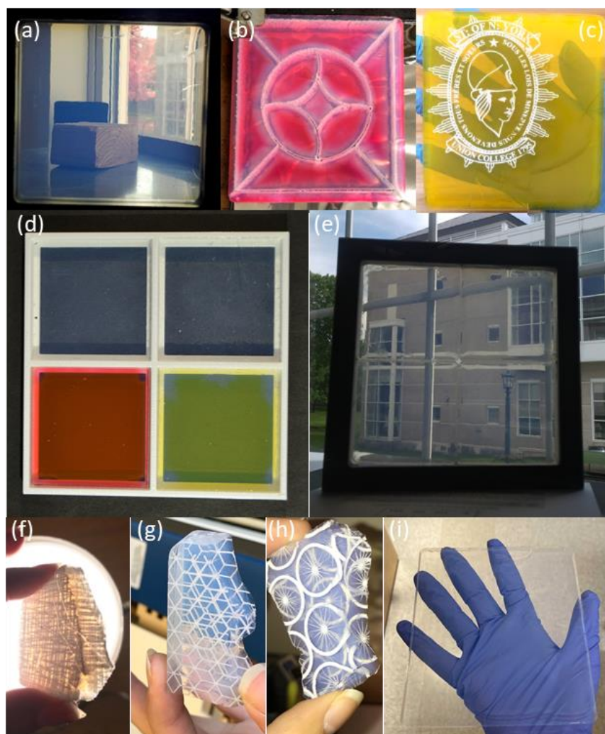
Figure 4. Photo montage of various aerogel window projects: (a) view through an 8.9 x 8.9 x 1.3 cm aerogel; (b) 10 x 10 x 1.5 cm Rhodamine-B-doped aerogel with pattern cut through width of aerogel; (c) 10 x 10 x 1.5 cm fluorescein-doped aerogel with etched pattern on surface of aerogel; (d) view of a 2 x 2 style window prototype on black flocked paper with a variety of transparent plain and dye-containing aerogel monolith tiles, each of size 50 x 50 x 0.5 cm; (e) view through a 17.8 x 17.8 cm window prototype made from four 8.9 x 8.9 x 1.3 cm aerogel monoliths; (f), (g) and (h) various aerogel samples with patterns etched on front and back surfaces; and (i) transparent 13 x 12.5 x 0.5 cm aerogel monolith.
