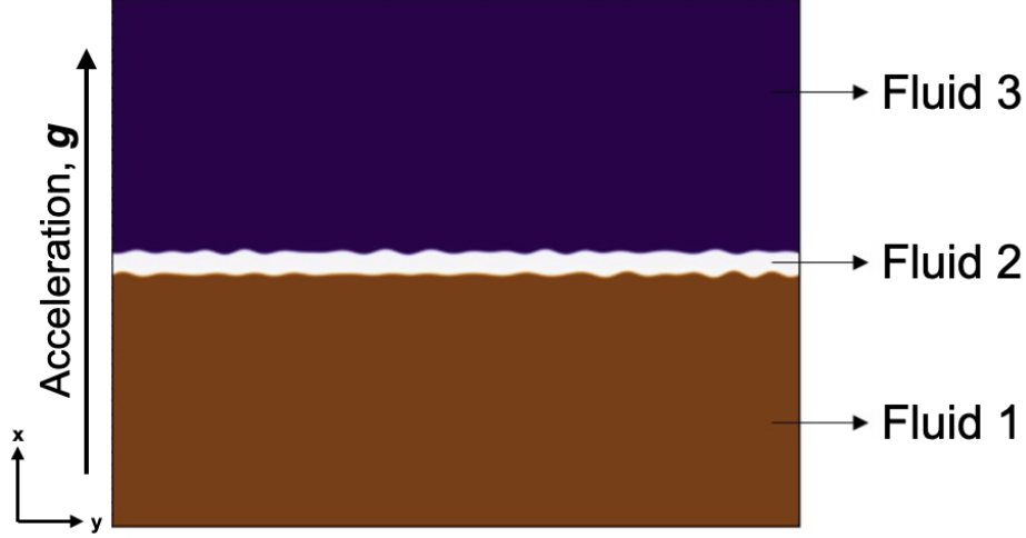
Fig. 1 Schematic visualization of three-layer RTI with three distinct fluids. The upward arrow represents the direction of the acceleration field.
