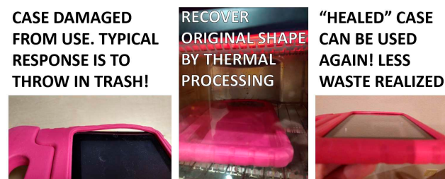
Figure 1. Using the inherent shape memory properties of EVA to enable the reuse of a damaged tablet case and reduce the amount of waste that would have been generated by throwing it away.
