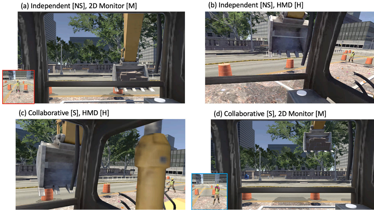
Fig. 8. FPV of the operator during the dumping operation: (a) Independent, 2D monitor trial (spotter stand in front of digging zone without sending any signals) (b) Independent, HMD trial (spotter stand in front of digging zone without sending any signals) (c) Collaborative, HMD trial (spotter stand in front of digging zone and was showing one hand signal) (d) Collaborative, 2D monitor trial (spotter stand in front of digging zone and was showing one hand signal).
