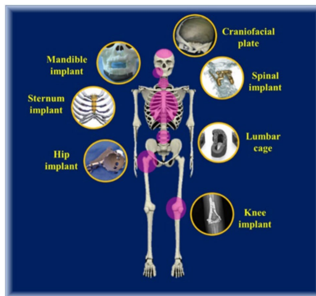
Fig. 3 3DP implants: craniofacial plate implant Ti-6Al-4V DMLS [64], mandibular implants [65], spinal [66] and sternum [67] implants, lumbar cage [68], hip [69], and knee implants [70]. Reprinted under copyright CC BY-NC-ND 4.0 license
