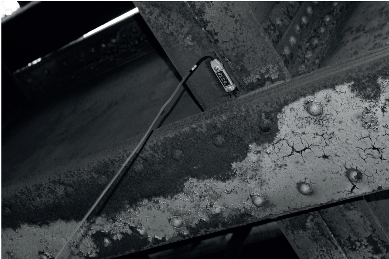
Fig. 5. Installed strain transducer on stringer bottom flange.
