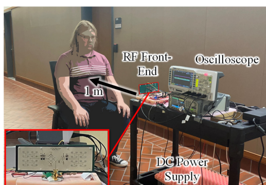
Figure 10. Respiration measurement setup. Target's chest is 1 m away from the radar system.
