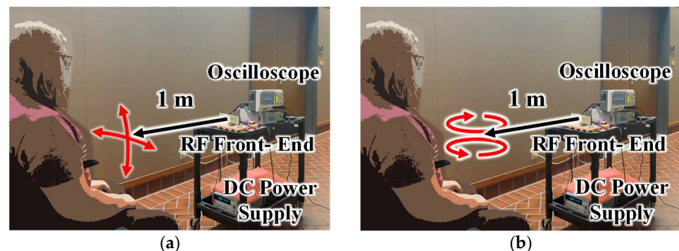
Figure 12. Gesture measurement setup for (a) up/down and left/right motion and (b) clockwise and counterclockwise rotation. Target's hand motions are approximately one meter away from the radar system for all tests.
