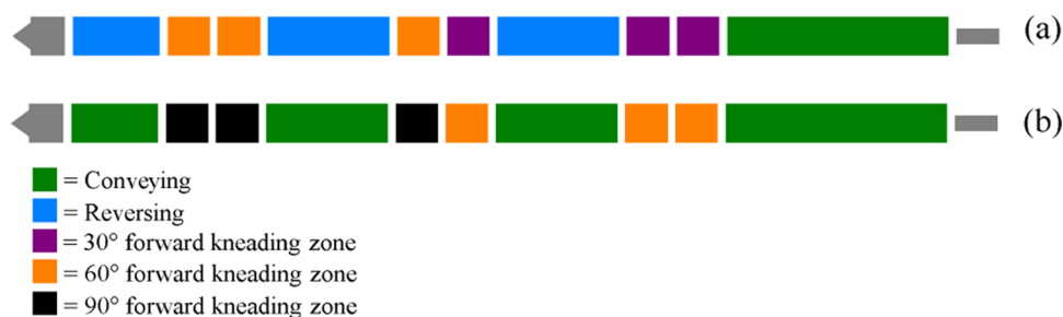
Figure 3. Illustration of Screw Configuration Comparisons for Nano 16 (a) and Process 11 (b) extruders (not to scale).
