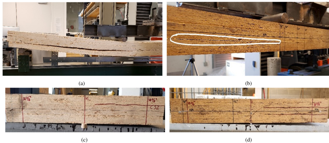
Fig. 14. (a) Four-point bending shear failure of a CLSVL beam ( l/h \geq 20 ) made of control strands, (b) premature glue line failure of four-point bending CLSVL beam ( l/h \geq 20 ) made of thermally modified strands, (c) three-point bending shear failure of a CLSVL beam ( l/h \leq 5 ) made of control strands, and (d) three-point bending shear failure of a CLSVL beam ( l/h \leq 5 ) made of thermally modified strands.
