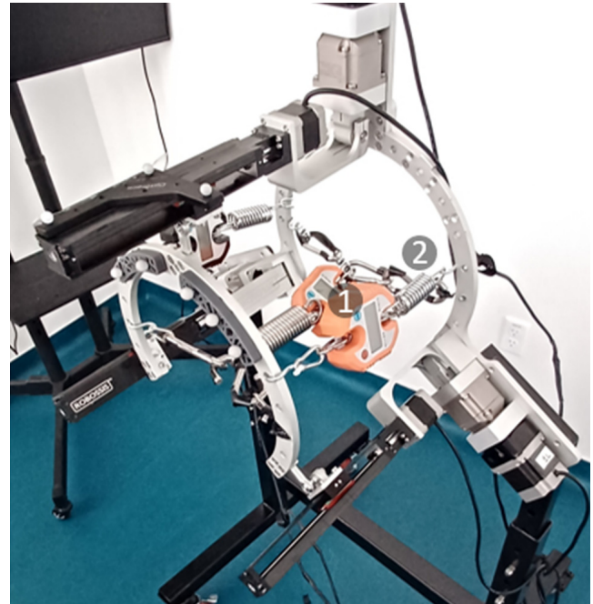
Fig. 6. The force testing benchtop model includes three force gauges (1) and three springs (2). Also, the force gauges and springs were attached to Robossis moving and fixed rings.
