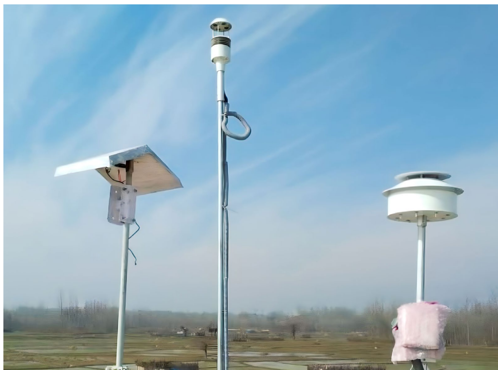
Fig. 3. General arrangements of APT maxima low-cost sensor and SASS sampler.
