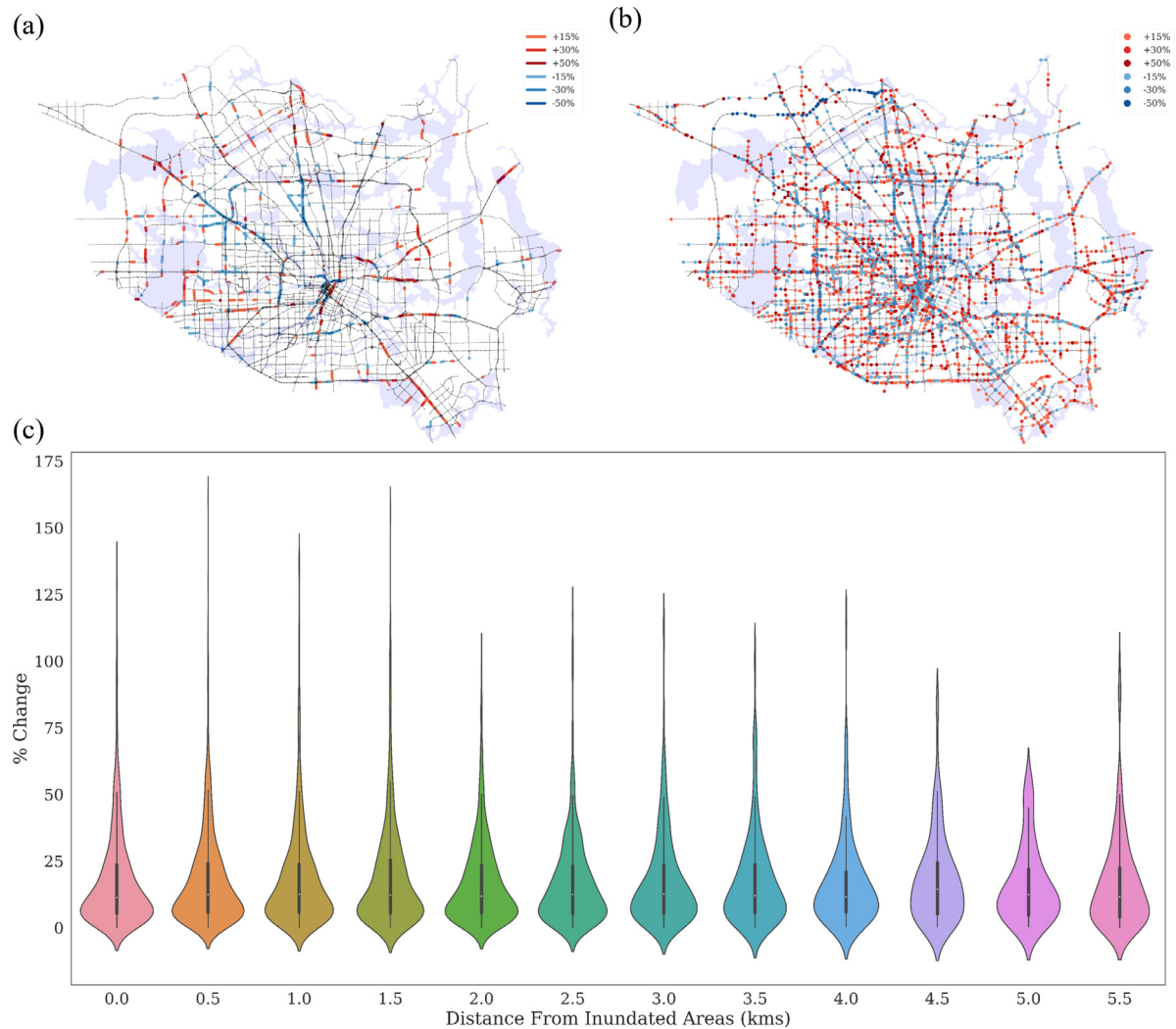
Fig. 6. Spatial impact of floods on traffic network on August 29. (a) Percent change in travel time for each road segment along with flooded regions for that day. (b) Average impact in terms of percent change in travel time at each node (road junction) when trips are considered to every other node. (c) Changes in travel time as a function of distance from flooded region. Change for regions within inundated region is shown by Violin plot at 0 distance; plot at 5.5 km distance presents the aggregated changes for all road junctions more than 5 km away, which accounts for less than 1% of the road junctions. There is no decay in change of travel time with respect to distance to inundated areas. Areas far from the flooded regions also show same extent of travel time change on an average.
