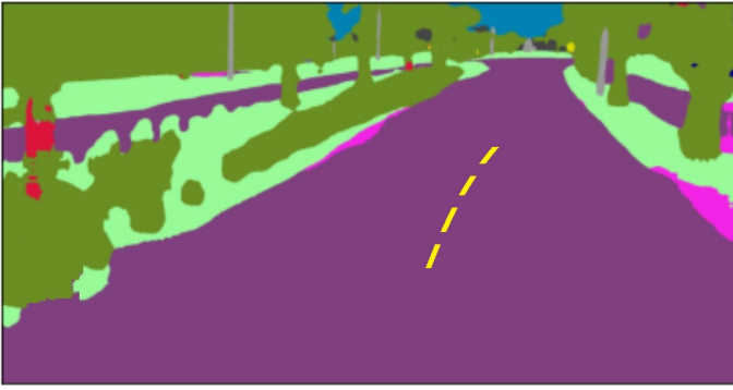
Figure 6. The yellow colored line is the automatically generated lane center. This is obtained by using the PSP-Resnet101 AI model, followed by a couple of more analytical openCV steps.
