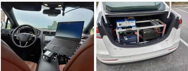
Figure 2. On the right, the Intel x86-64 laptop with NVIDIA GPU located inside the vehicle, and on the left a more powerful Intel x86-64 desktop with NVIDIA GPU, a SpeedGoat Mobile Real-Time target machine (Intel x86-64 based), and an a Samlex inverter located inside the trunk.
