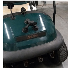
Figure 4. Forward looking camera with C-mount adapter for machine vision.
