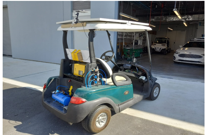
Figure 1. Drive-By-Wire capable Electric Golf-Cart demo video, https://www.youtube.com/watch?v=oRRvCas3oOU
