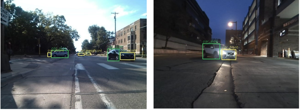
Fig. 5. Examples of the vehicle detection system on experimental images. The output of the YOLOv4-tiny is shown as yellow and green bounding boxes for car_front and car_side classes respectively.
