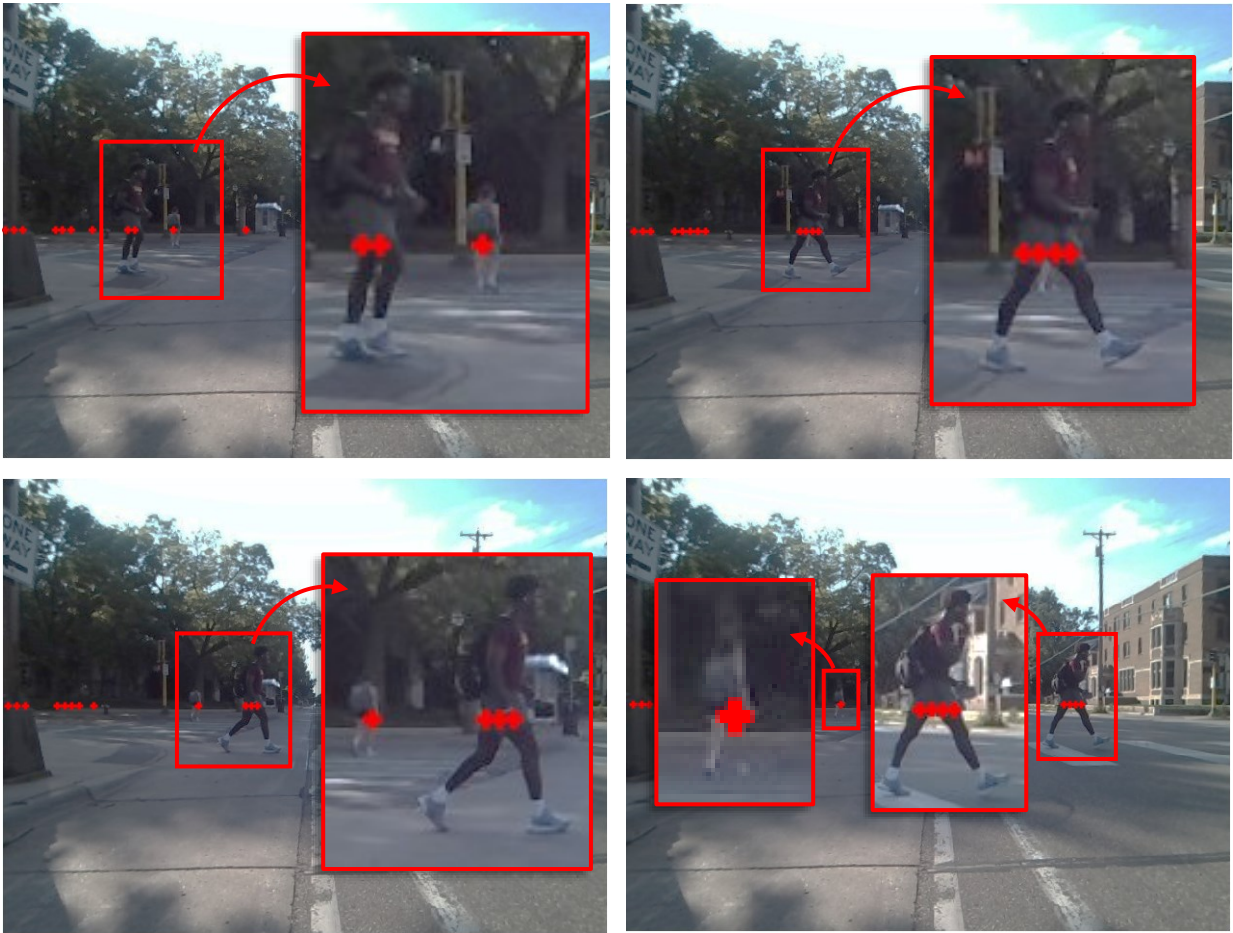
Fig. 3. LIDAR measurement points (shown as red crosses) and images are synchronized such that the measurements accurately lie on the pedestrians.
