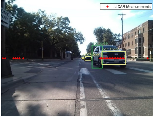
a) LIDAR and camera information before LIDAR- camera fusion.
