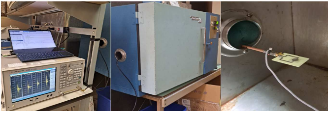
Fig. 3. (left) PC running a MATLAB script to control the VNA and (middle) PID controlled Tenney ETC. (right) PCB test fixture and LT sample inside the ETC.
