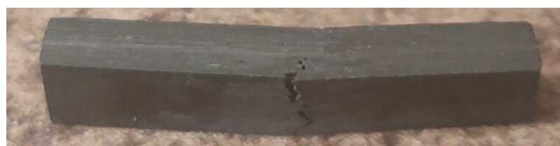
Figure 13. The SBS test of a ZT-CFRP/MCFA-AM sample showed the fiber-tensile-failure mode on the lower half section of the laminate instead of the expected standard delamination-failure mode.
