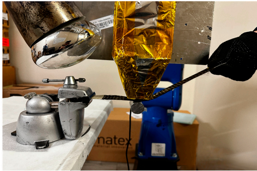
Figure 6. Illustration of the under-development robot-arm-driven MCFA-AM printer: a tape-like feedstock or filament (e.g., CFRP prepreg or ZT-CFRP prepreg) is hand-fed (the mechanical feeder is under development) and held in place by a backing article (metallic rod) attracted by a proprietary magnetic field emitter (sheathed with aluminum foil), with a heat lamp (not turned on in this illustration) pointing at the compaction region.
