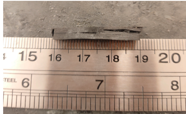
Figure 8. Cross section cut of a no-pressure-3DP CFRP laminate.
