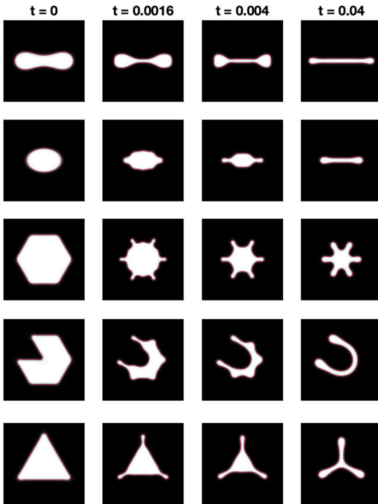
Fig. 12 Shape evolution of other shrinkage examples with different initial morphology but same parameters as those used in Fig. 10. They have a similar pattern: the inner region shrinks for the decline of osmotic energy and the sharp corners shrink to form finger-like structure; the shrinking process is with preserved surface area and mass; the concentrations of the inner and outer phases evolve to the corresponding equilibrium values
