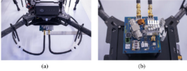
Fig. 18. Photographs of the HF-IPT transmitter on the Matrice 100 drone. (a) Transmit coil. (b) HF-IPT inverter board.
