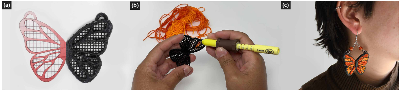
Figure 1: PunchPrint supports the creation of programmable and robust 3D-printed foundation textiles that are compatible with punch needle crafting. We present a design tool and fabrication workflow that reduces labor while supporting the production of detailed composite artifacts. Here we show how PunchPrint enables crafting small detailed designs. (a) We provide a parametric design interface for fabricating a flexible, filament-based textile substrate with design guides and hooks to facilitate assembly; (b) The craftsperson inserts fiber elements using standard punch needle embroidery methods on the 3D-printed foundation fabric; (c) The assembled final artifact with earring hooks and beads.
