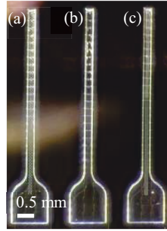
Figure 4. IP-S fabricated open microchannels with (a) micro diamonds, (b) control, and (c) micro ribs.
