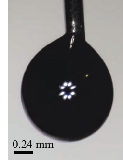
Figure 5. PEDOT:PSS primed at tip of needle for placement on pad areas.
