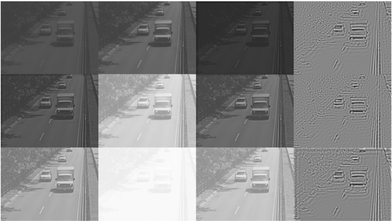
Fig. 7 Comparison between DNP processed images at 3 different brightness levels. (1st column) Input image. (2nd column) Output of the DNP without global feedback. (3rd column) Output of the DNP
