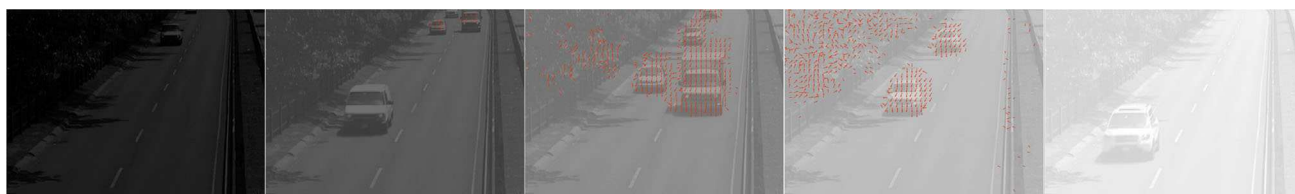
Fig. 3 Motion detection applied onto the same video sequence as in the second row of Fig. 2 after preprocessing by a sigmoidal function. The motion detector can no longer detect motion at very low and very high brightness levels
