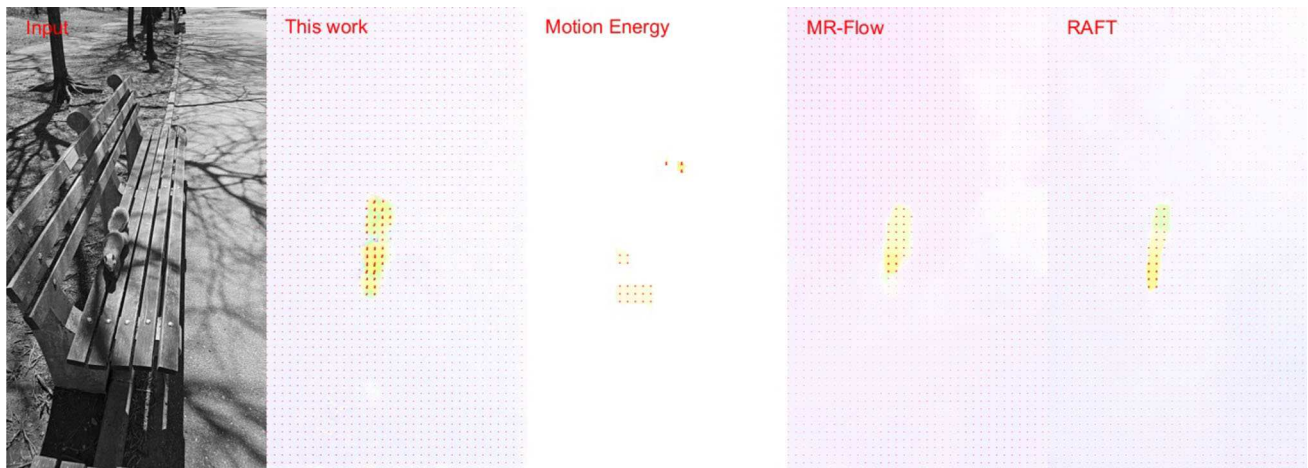
Fig. 9 Comparison of motion detected in a visual sequence shot at 240 fps. (1st column) A sample frame of a 240 fps visual sequence. (2nd column) Motion detected by the phase-based motion detector. (3rd column) Motion detected by the motion energy algorithm (Shi and Luo 2018). (4th column) Motion detected by the MR-Flow algorithm (Wulff et al.
